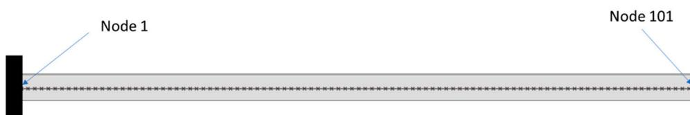
Figure 4. Mesh of the 100-element beam.
