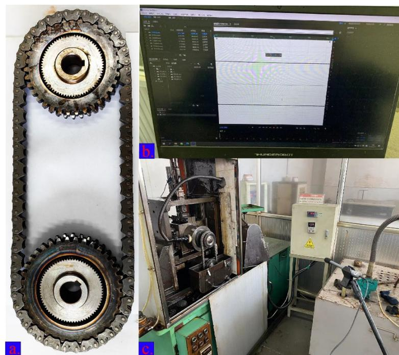
**Figure 2.** Noise test ((a) The Hy-Vo chain transmission system, (b) audio sampling, (c) the measurement microphone).
