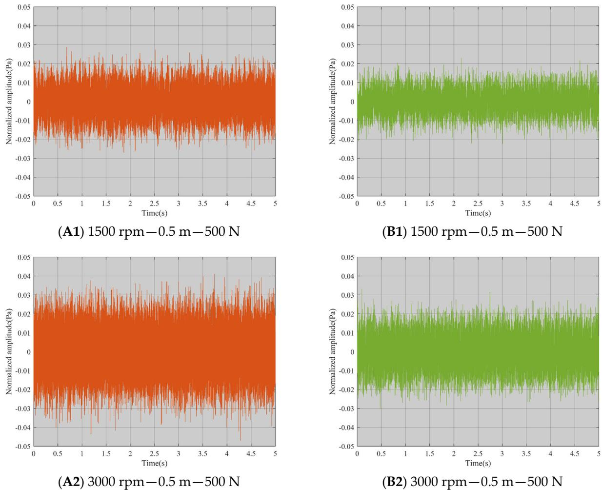
**Figure 3.** Time-domain waveform ((A1,A2) Hy-Vo chain system, (B1,B2) silent chain system).
