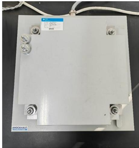
**Figure 1.** Physical diagram of the Epstein square ring.
