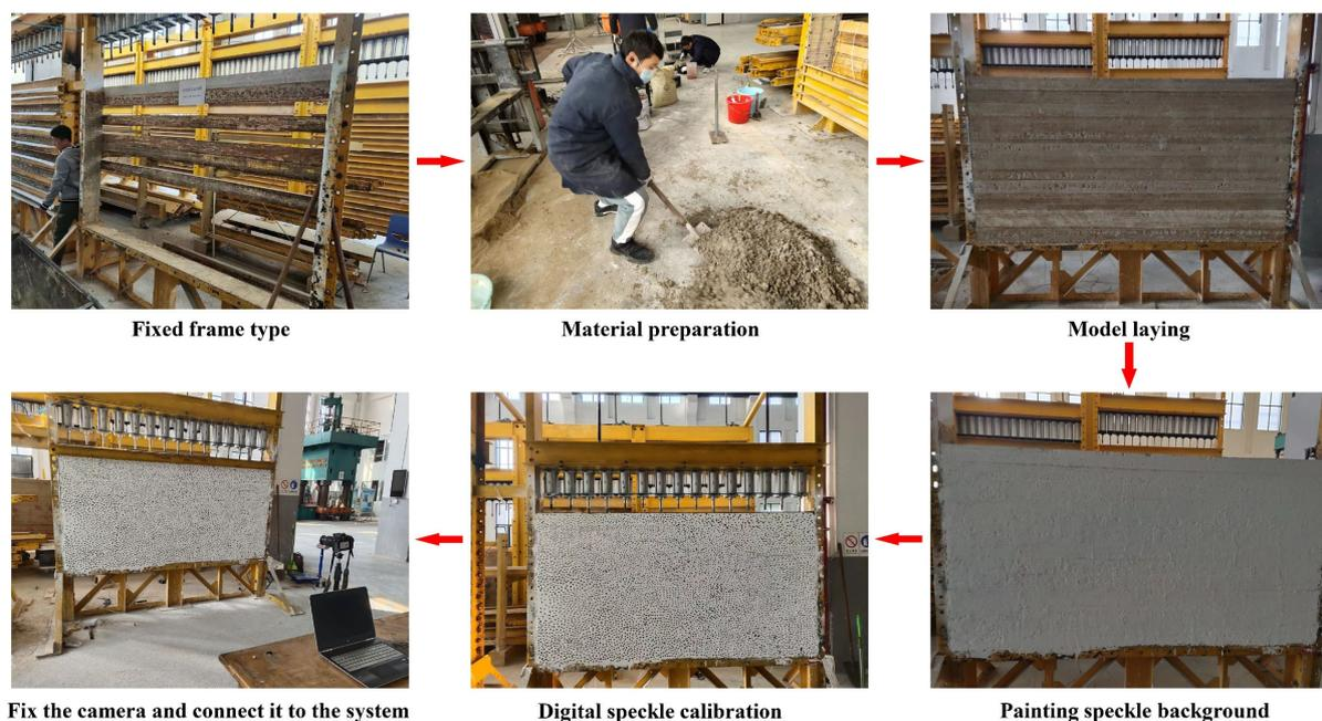
**Figure 3.** The figure shows the laying process for the physical similarity models.
