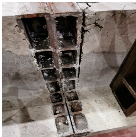
Figure 7. Flange connection failure diagram.
