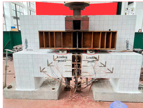
Figure 2. Schematic diagram of the flexure test loader.
