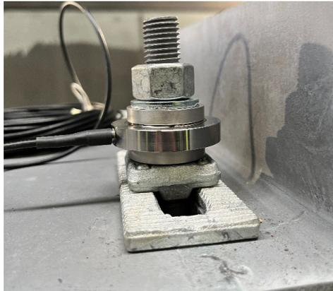
**Figure 13.** Zoom on the force washer installed on the bracket's bolt.
