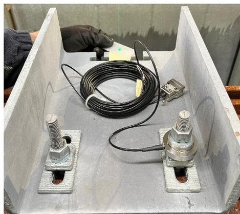
**Figure 14.** Façade bracket with force washer installation.
