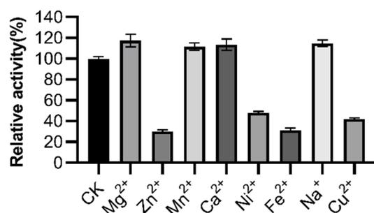
**Figure 5.** Effects of metal ions on LipGt6 activity. The enzyme was subjected to activity assays after treatment with 5 mM metal ions ( $Zn^{2+}$ ,  $Mg^{2+}$ ,  $Ca^{2+}$ ,  $Mn^{2+}$ ,  $Cu^{2+}$ ,  $Ni^{2+}$ ,  $Fe^{2+}$ , and  $Na^+$ ) for 1 h at 50 °C. The relative activity of the control without metal ions was regarded as 100%. Data points are the average of triplicate experiments, and error bars represent standard deviation.
