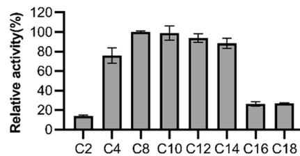
**Figure 3.** Substrate specificity of recombinant LipGt6. Reactions were incubated at 50 °C with 50 mM Tris-HCl buffer, pH 9.0. C2, *p*NP-C2; C4, *p*NP-C4; C8, *p*NP-C8; C10, *p*NP-C10; C12, *p*NP-C12; C14, *p*NP-C14; C16, *p*NP-C16; C18, *p*NP-C18. Data points are the average of triplicate experiments, and the bars indicate the standard deviations.
