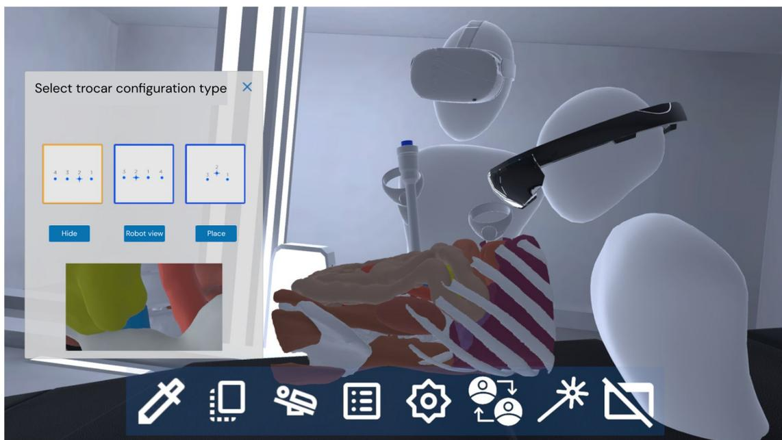
**Figure 7.** Virtual trocar tool, with which users in VR mode can freely position the trocar directly with 6-DOF VR controllers. As in the XR case, all participants in the room can visualise in real time the first-person view of the robot that would be obtained thanks to the trocar pose.
