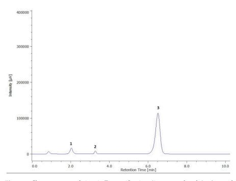
**Figure 1.** Chromatogram of vitamin E quantification.  $(1-\alpha$ -tocopherol;  $2-\beta$ -tocopherol; 3—tocol-internal standard).
