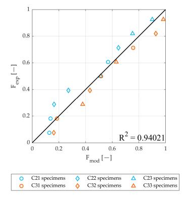
**Figure 3.** Probability–probability diagram of the estimated CDF ( $F_{mod}$ ) versus the experimental empirical CDF ( $F_{exp}$ ) for the 24 mm wide (in blue) and 36 mm wide specimens (in orange). The coefficient of determination,  $R^2$ , of the least squares fit of the bisector to the points is also shown.
