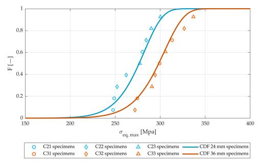
**Figure 4.** Model cumulative distribution function of the maximum equivalent stress for the 24 mm and 36 mm specimen types. Experimental observations are shown as individual markers.
