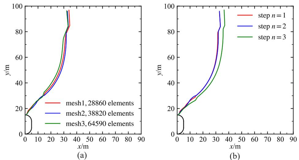
**Figure 13.** Variation in potential fracture surfaces with mesh and computational step for silo-type caverns overlying rock masses under Class III rock mass ( $K = 0.5$ ): (a) the number of mesh elements; (b) the computational step length
