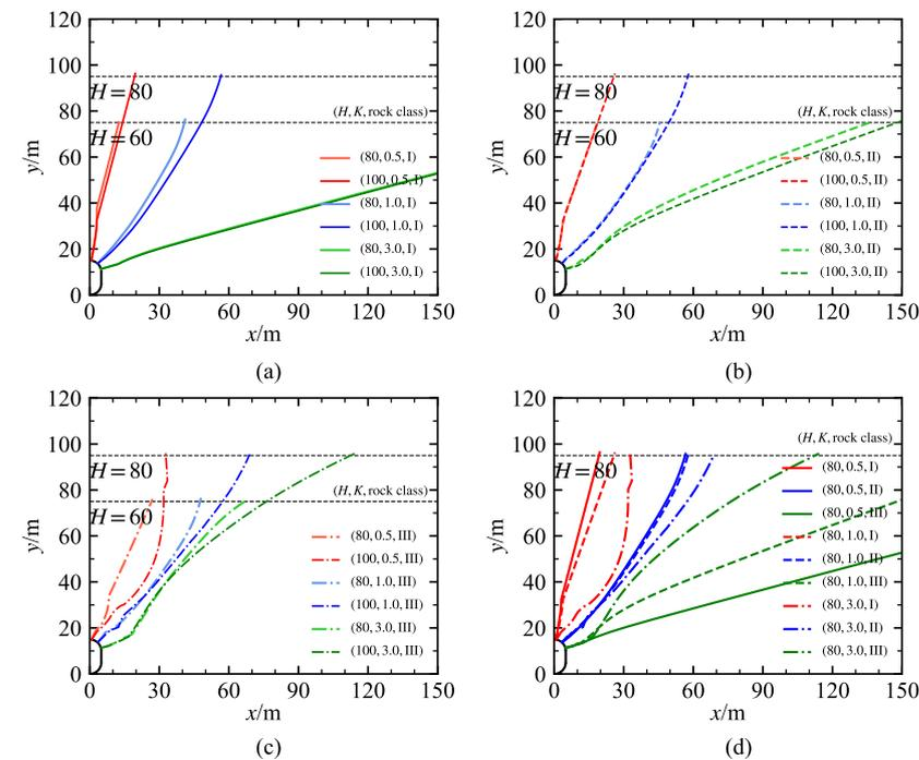
**Figure 9.** Potential fracture surfaces in different rock grades of silo-type LRCs: (a) Class I rock mass; (b) Class II rock mass; (c) Class III rock mass; (d) comparison of different rock grades (burial depth of 80 m).
