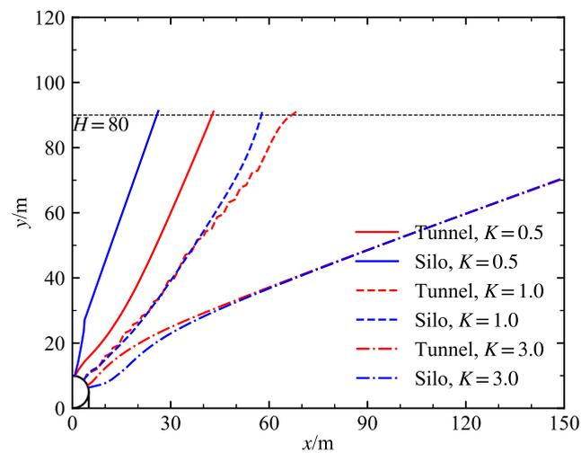
**Figure 11.** Potential fracture surfaces for different types of LRCs in the Class II rock mass (burial depth of 80 m).
