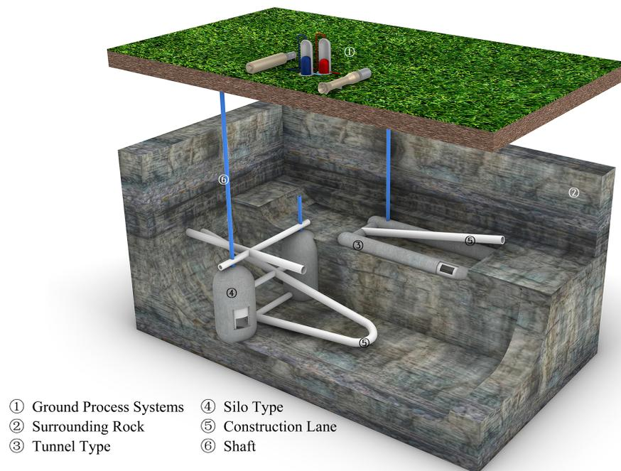
**Figure 3.** The key problems and main structure of an LRC.
