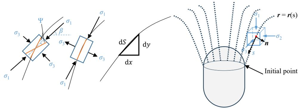
Figure 6. Schematic diagram of potential fracture surface solution.
