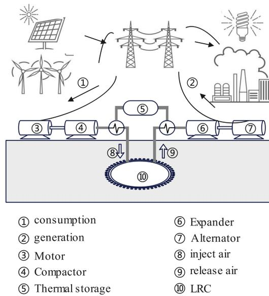
**Figure 1.** The working principle of CAES.
