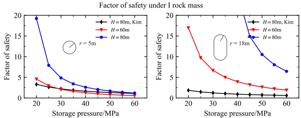
Figure 14. Factors of safety for tunnel- and silo-type LRCs under Class I rock at different burial depths.
