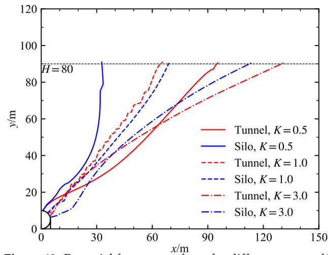
**Figure 12.** Potential fracture surfaces for different types of LRCs in the Class III rock mass (burial depth of 80 m).
