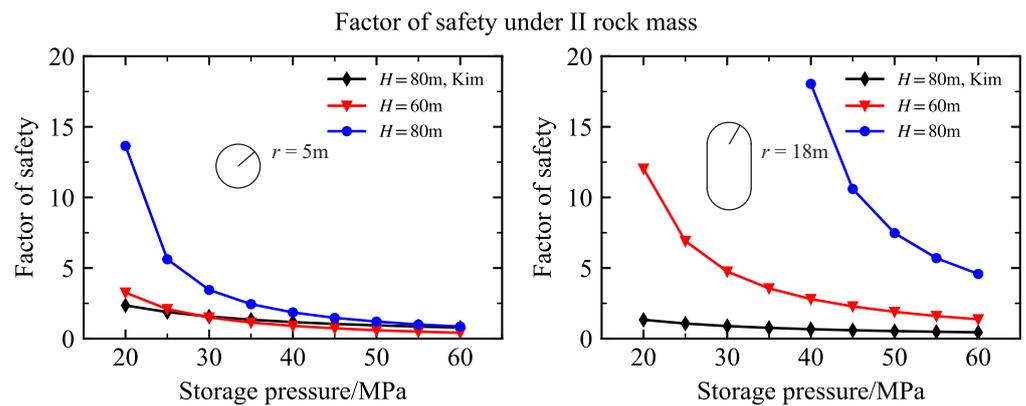
Figure 15. Factors of safety for tunnel- and silo-type LRCs under Class II rock at different burial depths.
