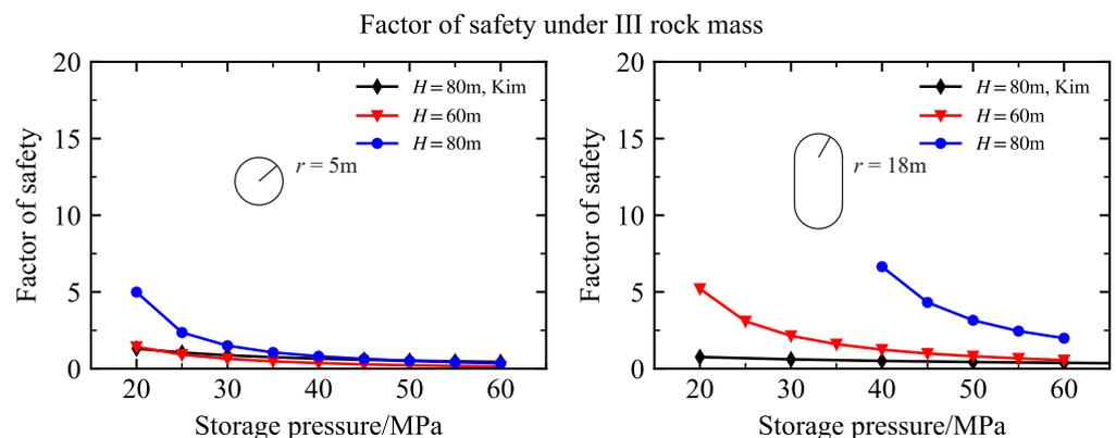
Figure 16. Factors of safety for tunnel- and silo-type LRCs under Class III rock at different burial depths.
