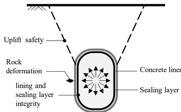
**Figure 2.** The key problems and main structure of an LRC.
