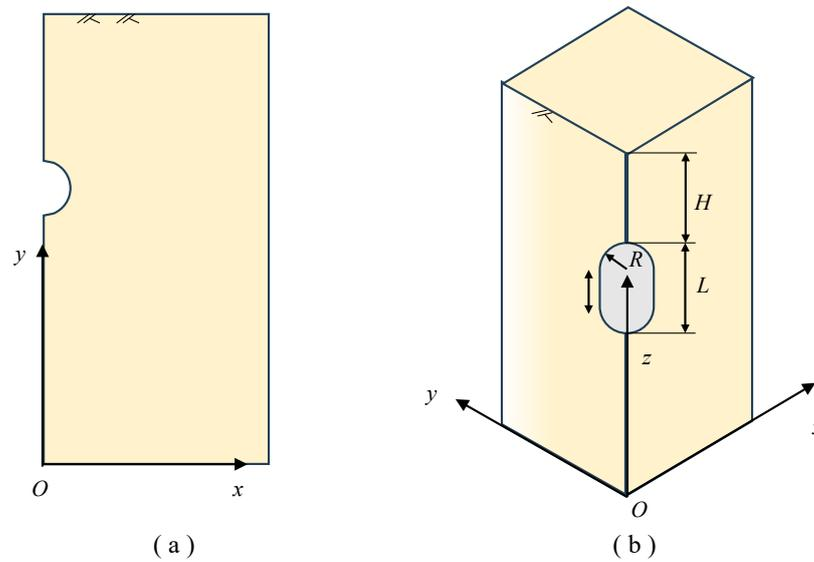
**Figure 5.** Schematic diagram of the computational model: (a) tunnel-type; (b) silo-type.
