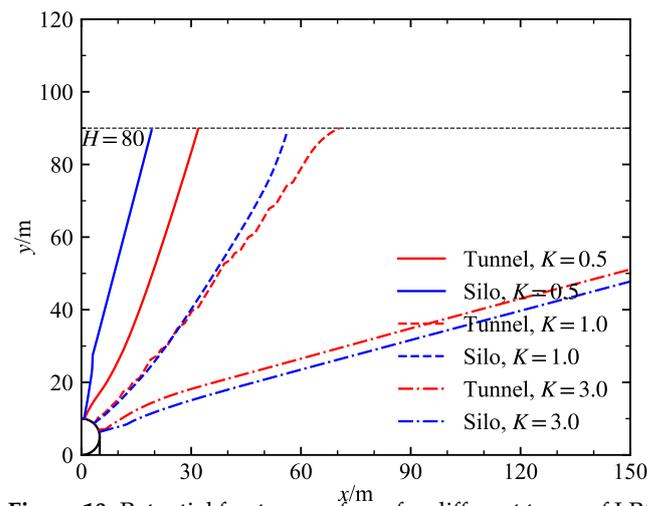
**Figure 10.** Potential fracture surfaces for different types of LRCs in the Class I rock mass (burial depth of 80 m).
