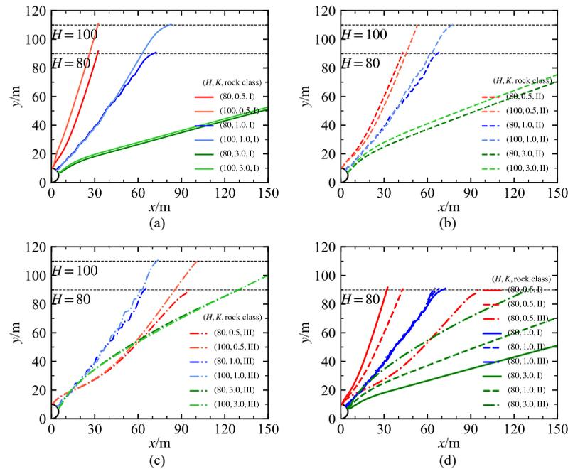
**Figure 8.** Potential fracture surfaces in different rock grades of tunnel-type LRCs: (a) Class I rock mass; (b) Class II rock mass; (c) Class III rock mass; (d) comparison of different rock grades (burial depth of 80 m).
