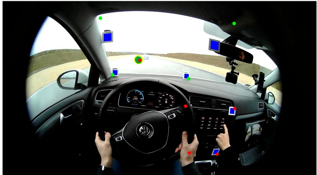
**Figure 7.** Incorrect recognition of the dashboard area-gaze position (yellow circle with green fill), detected tags (blue squares), compensated tag positions (dots in the corners) and “gaze on dashboard” indication (red dots).
