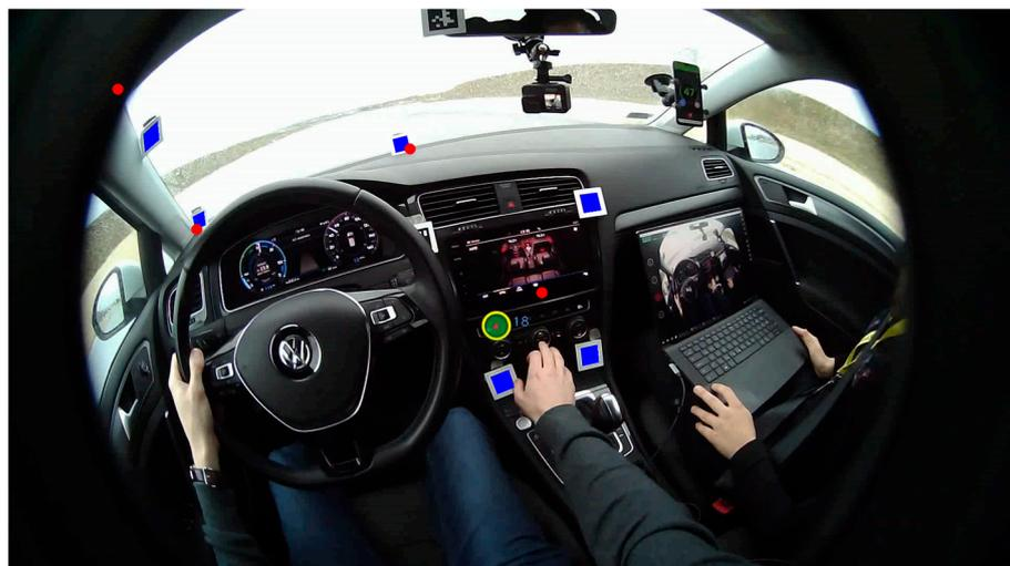
**Figure 6.** Gaze position (yellow circle with green fill), detected tags (blue squares), compensated tag positions (dots in the corners) and “gaze-on-road” indication (dots are red not green).
