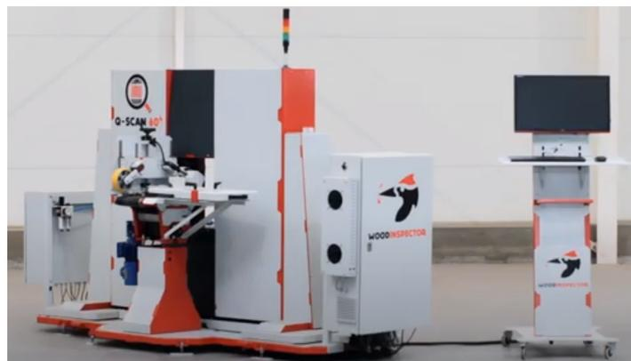
**Figure 1.** A Q-scan 60 system, which implements a blue stain detection algorithm using neural networks.
