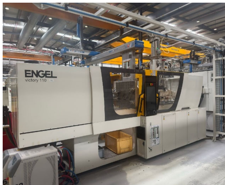
Figure 3. Injection machine selected for the SMED Workshop (front view)—Machine D.
