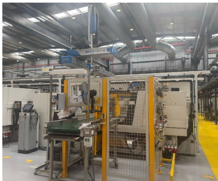
Figure 4. Injection machine selected for the SMED Workshop (rear view—operator area)—Machine D.
