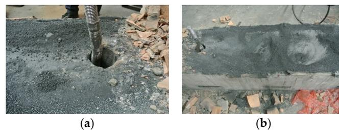
Figure 14. MG slide and restrictive rebars upon failure of wall (a) buckled restrictive rebars; (b) MG slide upon failure of wall.
