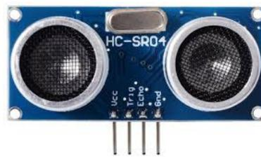
Figure 13. Ultrasonic sensors.
