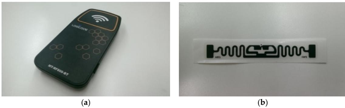
Figure 16. (a) Ultra High Frequency (UHF) RFID reader MT-RF800-BT and (b) UHF tag.
