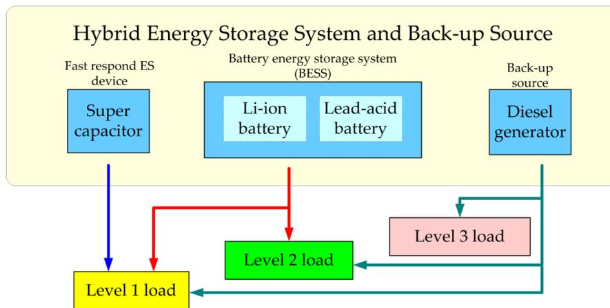
**Figure 4.** Principle of source-load coordination. ES, energy storage.
