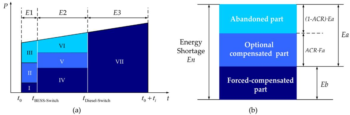
**Figure 7.** Illustration of discharge strategy with additional compensation ratio (ACR) considered. (a) Stages of energy shortage; (b) Three parts of an energy shortage stage. ACR, additional compensation ratio.
