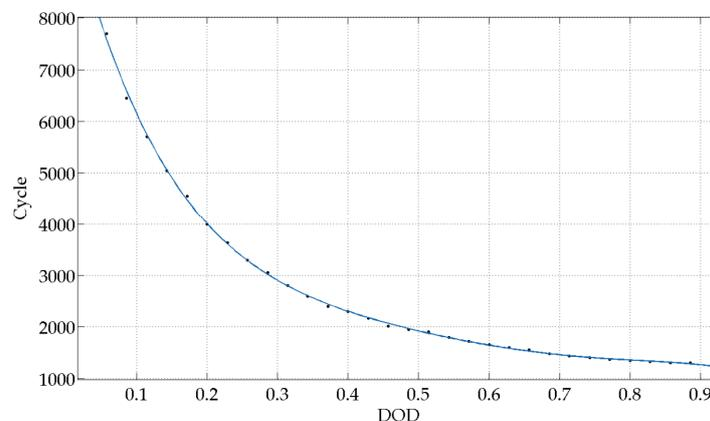
**Figure 2.** Cycle time of lead-acid batteries. DOD, depth of discharge.
