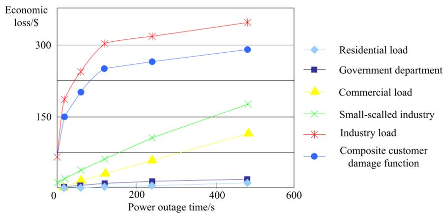
**Figure 3.** Economic loss curve of typical load after power outage.
