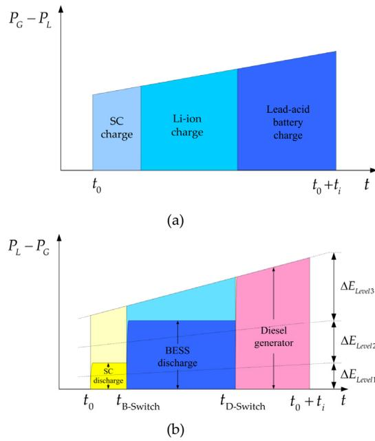
**Figure 5.** Operation status and coordination strategy of power sources in different conditions. (a) Illustration of charging process; (b) Illustration of discharging process. SC, super capacitor.
