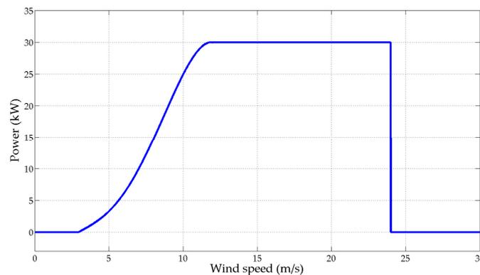
Figure 1. Power output curve of wind turbine (WT).
