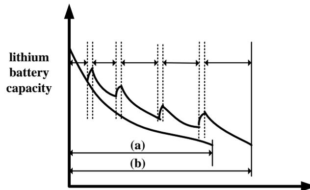
**Figure 2.** Lithium battery capacity changing with discharge process. (a) Continuous discharge; (b) intermittent discharge.
