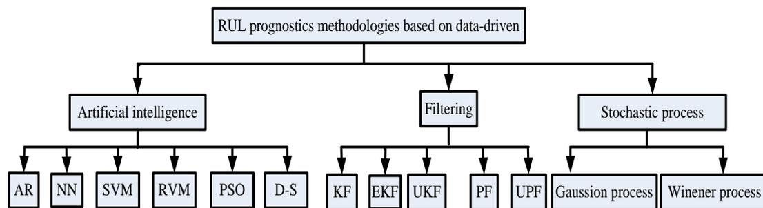
**Figure 1.** The main remaining useful life (RUL) prognostics methodologies of vehicle lithium-ion batteries.
