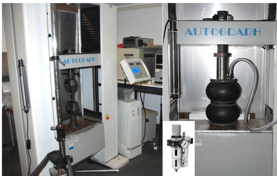
**Figure 10.** Mounting of the bellows pneumatic accessory in a SHIMADZU® testing machine between the working table and upper crosshead with an adaptor ram and a pressure air control unit.
