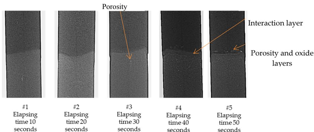
**Figure 2.** Sample interfaces EN AC 48000/EN AC 42100 obtained with RX analysis after sequential gravity casting at different conditions of waiting time. AlSi12CuNiMg is the dark grey part (the lower part for each image) while the other one is AlSi7Mg0.3.
