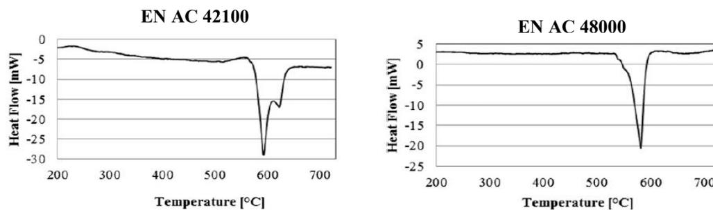
Figure 1. Differential Scanning Calorimetry (DSC) analysis [10].
