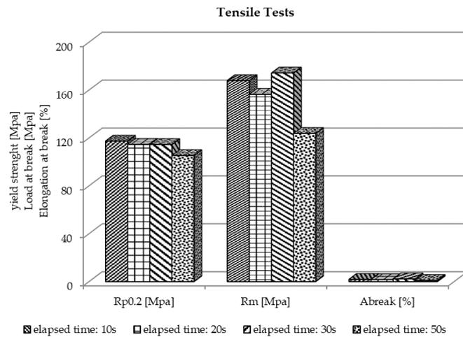
Figure 3. Mechanical properties obtained after tensile tests.
