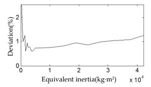
Figure 24. Simulated deviation of electrical inertia.
