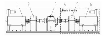
1 electric motor, 2-reducer, 3-reducer, 4 - torque sensor, 5 - reducer, and 6 - tested motor.
