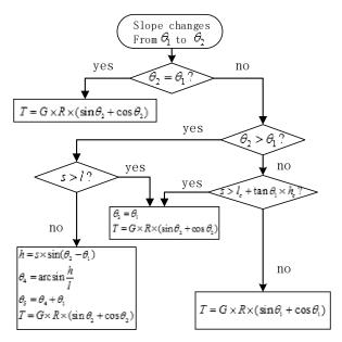
Figure 4. Chart of car body inclination angle and resistance moment analysis.
