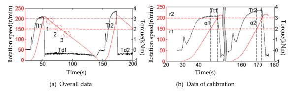
**Figure 16.** Calibration test results under equivalent inertia of 2227.84 kg·m<sup>2</sup>.
