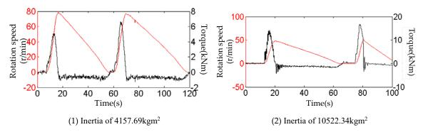
Figure 23. Calibration test results under equivalent inertia of 4157.69 kg·m<sup>2</sup> and 10,522.34 kg·m<sup>2</sup>.
