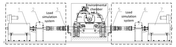
1 - electric motor, 2 - reducer, 3 - torque meter and encoder, 4 - tested vehicle, 5 - torque meter and encoder, 6 - reducer, 7 - electric motor.
