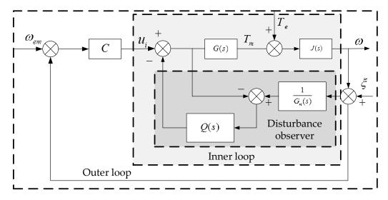
Figure 11. Control loop with a disturbance observer.
