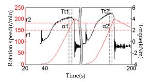
**Figure 17.** Calibration test results under equivalent inertia of 4177.2 kg·m<sup>2</sup>.
