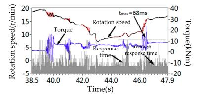
**Figure 27.** The system response time under the preset path spectrum.
