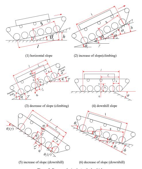
Figure 3. Force analysis of a tracked vehicle.
