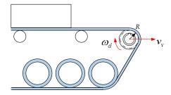
Figure 5. The relationship between body speed and driving wheel speed.
