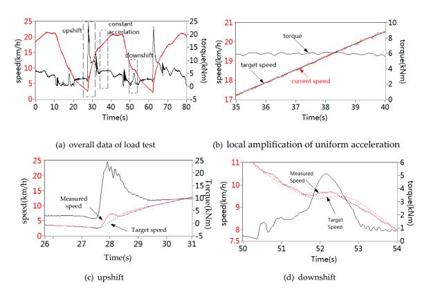
Figure 29. Load and shift test.
