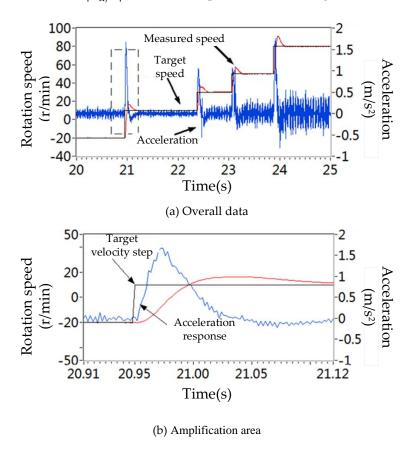
Figure 25. Electrical inertia response time at constant torque.
