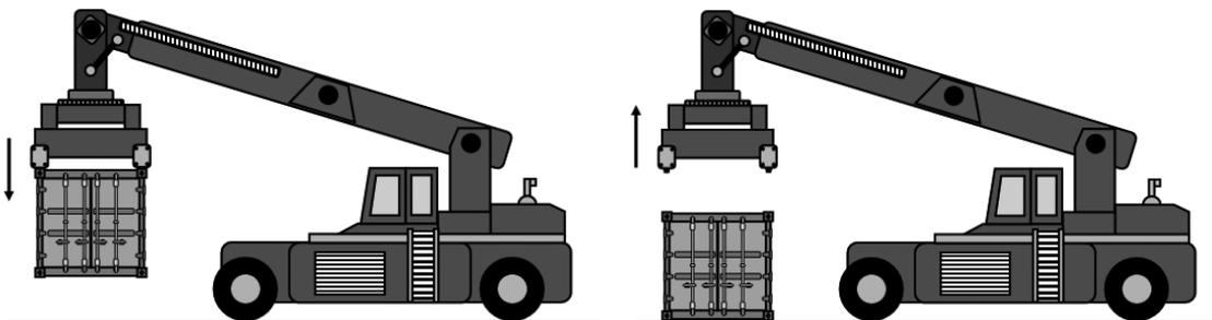
**Figure 2.** Operation No. 2—setting aside a large type A container on a first layer stack (ground), within a prescribed sector of a storage yard. Source: own work.
