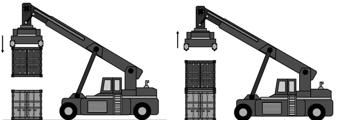
**Figure 3.** Operation No. 3—setting aside a large type A container on a second layer stack, within a prescribed sector of a storage yard. Source: own work.
