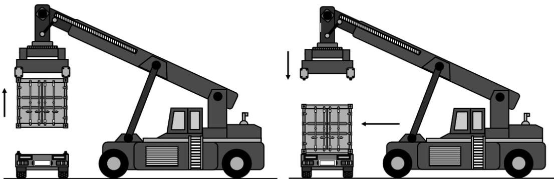
**Figure 1.** Operation No. 1—raising a large type A cargo container from a tractor-trailer. Source: own work.
