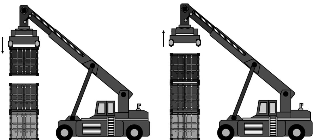
**Figure 4.** Operation No. 4—setting aside a large type A container on a third layer stack, within a prescribed sector of a storage yard. Source: own work.
