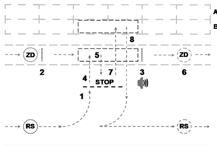
**Figure 5.** The scheme of a transportation cycle: from picking up of a large type A container from a tractor-trailer by a reach stacker to setting it aside in a prescribed storage area. Source: own work.
