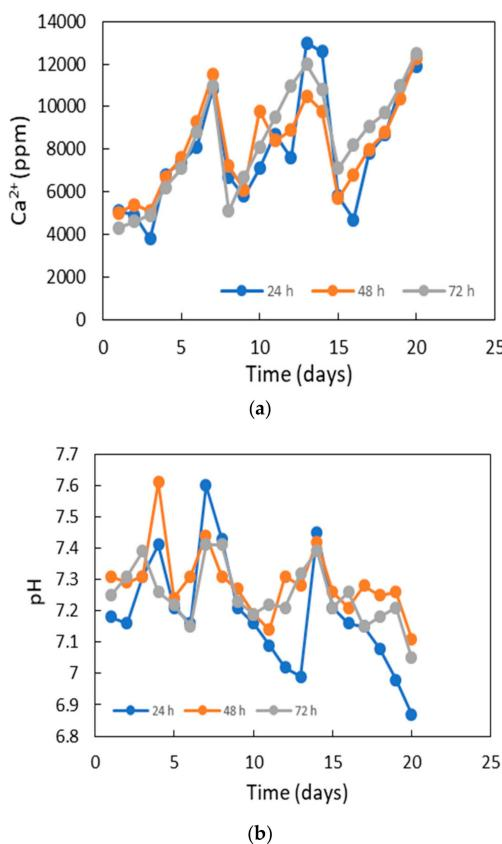
**Figure 8.** (a) Temporal variation of Ca<sup>2+</sup> and (b) pH in the effluent from solidification solution in days.
