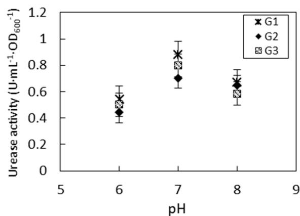
**Figure 4.** Impact of pH for the urease activity of the reaction solution at  $30\text{ }^{\circ}\text{C}$ .
