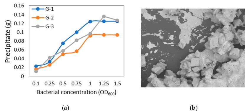
**Figure 7.** (a) CaCO<sub>3</sub> precipitation trend of the isolated strains and (b) SEM images of the precipitated CaCO<sub>3</sub> of G1 species.
