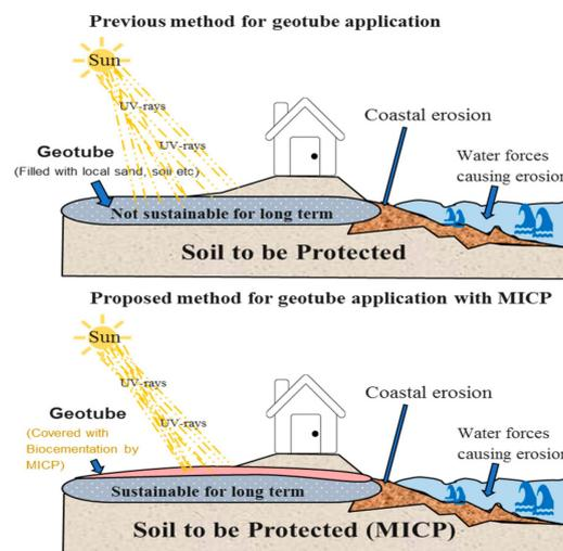
Figure 10. Proposed coastal erosion protection method.
