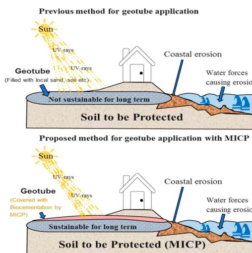
**Figure 10.** Proposed coastal erosion protection method.
