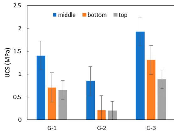
**Figure 9.** Comparison of estimated unconfined compressive strength (UCS) in each strain.
