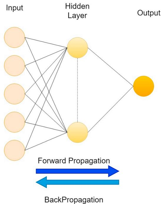
**Figure 1.** Typical structure of backpropagation algorithm-artificial neural network (BP-ANN) algorithm.
