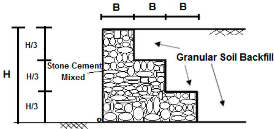
Figure 4. Dimension model for gravity masonry retaining wall.
