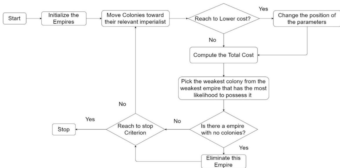
**Figure 3.** Structure of the imperialist competitive algorithm (ICA) algorithm.
