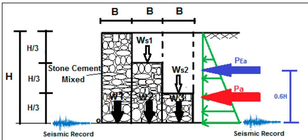
Figure 5. Distribution of active force for static and dynamic conditions with body forces for soil and Stone blocks.
