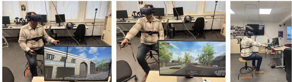
**Figure 7.** Picture of the laboratory setup. Staged pictures (left to right) of a participant performing a VR exploration session and the pointing north task. The picture on the right shows the experimental setup from the side, including the swivel chair and cable management system.
