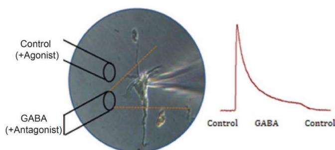
**Figure 1.** Application of solutions using capillaries. The application of solutions was controlled using solenoid valves; on the right of the photo, there is a representative trace of the current generated by the GABA application.
