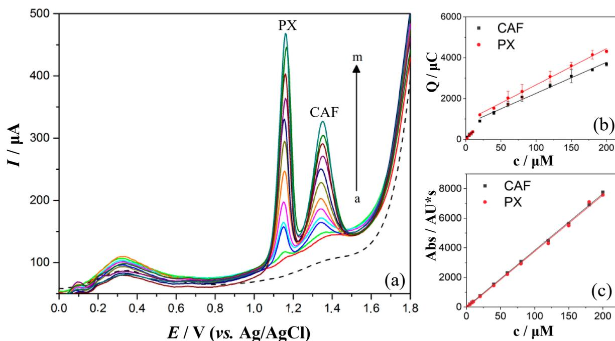
**Figure 4.** (a) DP voltammograms of equimolar mixtures of paraxanthine (PX,  $E_{PX} = +1.15$  V) and caffeine (CAF,  $E_{CAF} = +1.36$  V): blank, 1, 2, 5, 8, 20, 40, 60, 80, 120, 150, 180 and 200  $\mu\text{M}$  in 0.1 M  $\text{H}_2\text{SO}_4$  on the GC electrode at a scan rate of  $5 \text{ mV s}^{-1}$ ; corresponding calibration curves by (b) differential pulse voltammetry (DPV) and (c) UHPLC-UV.
