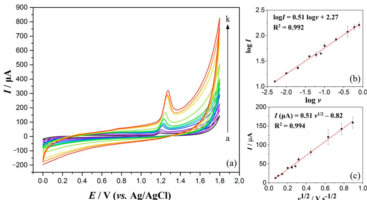
**Figure 3.** (a) Cyclic voltammograms of 400  $\mu\text{M}$  PX at various scan rates (from a to k): 5, 10, 20, 40, 60, 80, 100, 200, 400, 600 and 800  $\text{mV s}^{-1}$  in 0.1 M  $\text{H}_2\text{SO}_4$  on the GC electrode; (b)  $\log I$  against  $\log \nu$ ; (c)  $I$  against  $\nu^{1/2}$ .
