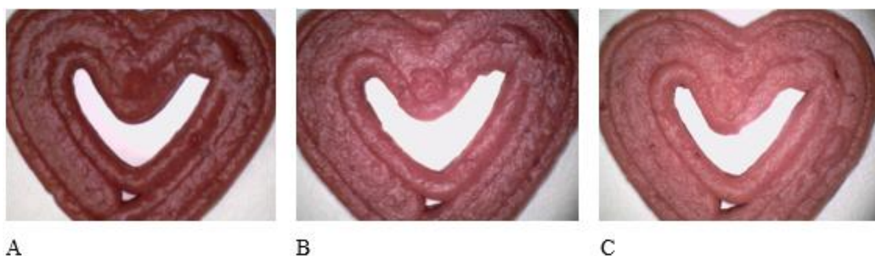
Figure 1. Microscopic pictures (500 \times ) of 3DP samples: Influence of added starch, 10% (A); 15% (B); 20% (C), on the lightness ( L^* ).
