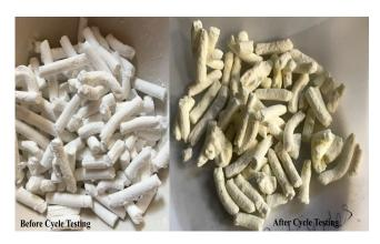
Figure 4. Photographs of the adsorbent pellets before and after the cyclic testing.
