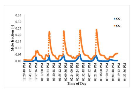
**Figure 14.** AR B CO and CO<sub>2</sub> exit composition.
