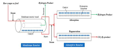
**Figure 1.** The schematic of the MR-AR Process.
