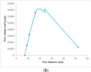
**Figure 5.** Pore size distribution of Batch #33 pellets: (a) Horvath–Kawazoe differential pore volume; (b) BJH adsorption dV/dD pore volume.
