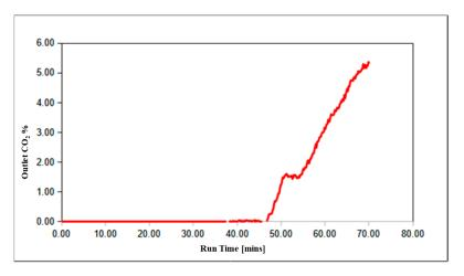
Figure 8. CO<sub>2</sub> breakthrough data from AR A unit during a combined MR-AR run at M&PT.
