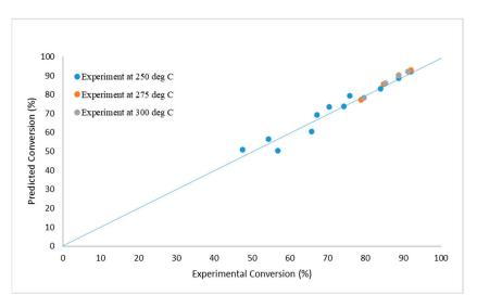
Figure 6. Kinetics data for catalyst #2, and parameter fit using the Associative mechanism.
