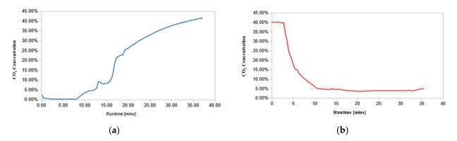
Figure 9. Experimental data for AR Run#4: (a) adsorption/reaction process; (b) regeneration process.
