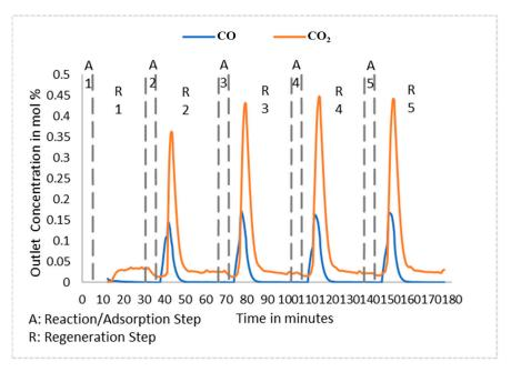
Figure 12. CO and CO<sub>2</sub> concentration in the AR A exit stream showing cyclic behavior.
