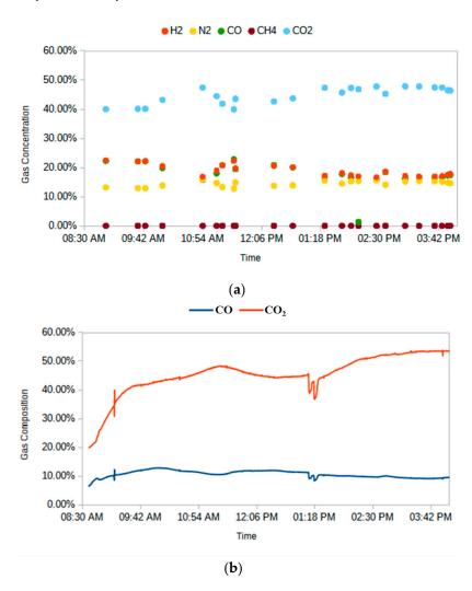
$\textbf{Figure 10.} \ \ \text{MR experiments: (a) syngas feed composition; (b) MR reject-side CO and CO_2 composition.}$
