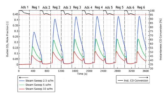
**Figure 3.** Outlet CO<sub>2</sub> mole fraction for different regeneration steam sweep rates (left vertical axis) and instantaneous CO conversion during adsorption phases (right vertical axis) at the AR outlet.
