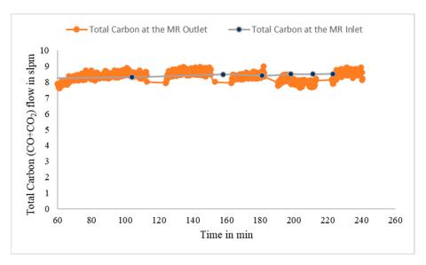
Figure 13. Total carbon (CO + CO<sub>2</sub>) flow in the MR inlet and MR reject-side exit.
