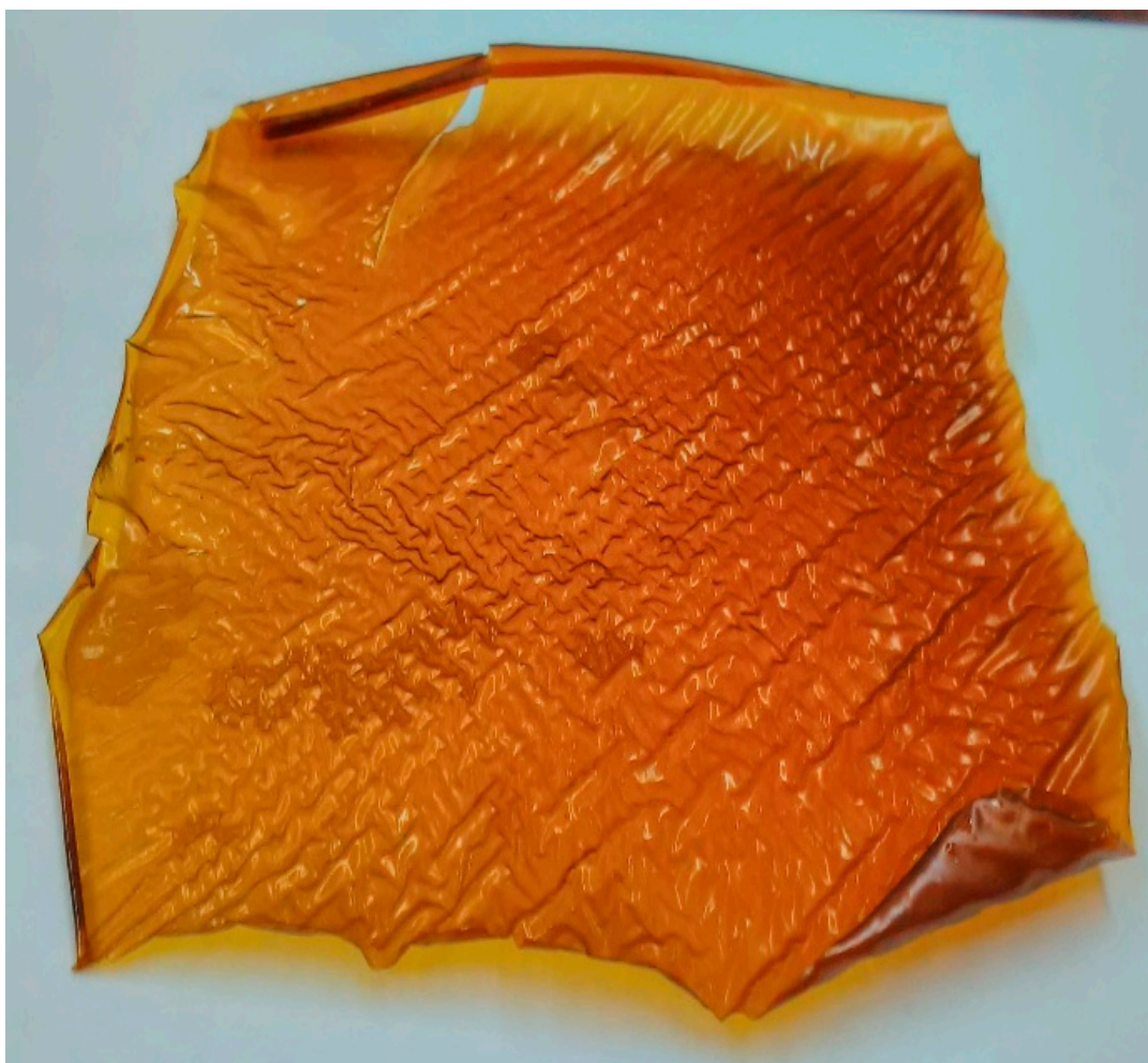
Figure S3. Image of membrane MHC4-C (2) after use in the EW cell. Which shows that the membrane ruptured during use.
