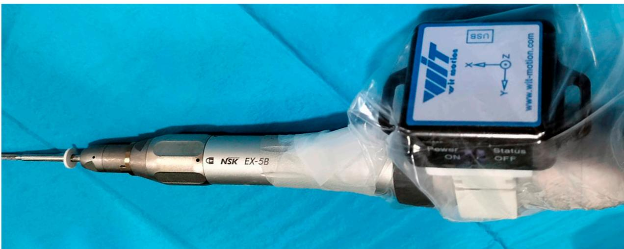
**Figure 3.** A goniometer incorporated to the surgical micromotor sends the data to a mobile phone via Bluetooth.
