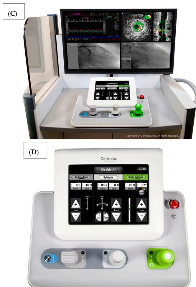
**Figure 1.** The CorPath GRX system. The robotic arm and disposable cassette is shown in (A). The arm extends freely from the table mount to allow variable configurations for catheter attachment (B). The interventional cockpit is shown in (C) with a close up of the workstation showing the joystick controls in (D). (Provided by and with permission from Corindus Vascular Robotics, Boston, MA, USA).
