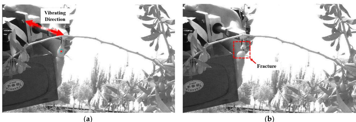
**Figure 7.** The process before the vibration (a) and under the vibration (b) recorded by the high-speed camera.
