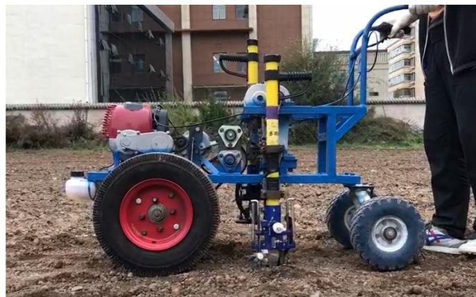
**Figure 22.** 2BZ-2 type cavity planter with vertical insertion.
