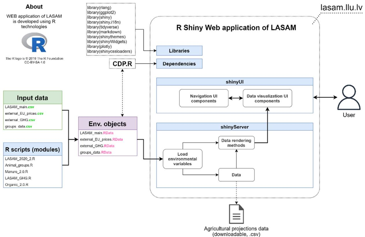
**Figure 2.** Architecture of the interactive WEB application of the LASAM model.
