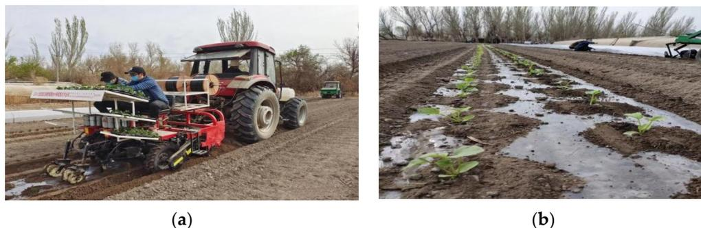
**Figure 4.** Field testing site. (a) Transplanter working test site. (b) The effect of transplanting cantaloupe.
