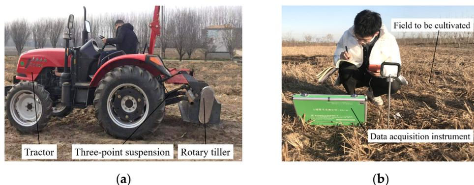
Figure 14. Field experiment. (a) Test device; (b) data acquisition.
