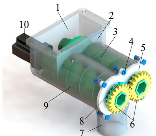
**Figure 1.** Schematic diagram of the double arc groove screw fertilizer discharger: 1. Fertilizer inlet. 2. Shell. 3. Left-handed fertilizer discharge wheel. 4. Bolt fertilizer discharge wheel. 5. End cover. 6. Gear. 7. Fertilizer outlet. 8. Direction of rotation. 9. Right-handed fertilizer discharge wheel. 10. Motor.
