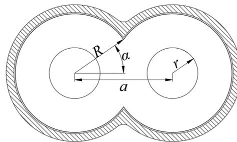
**Figure 4.** Schematic diagram of the inner cavity area.
