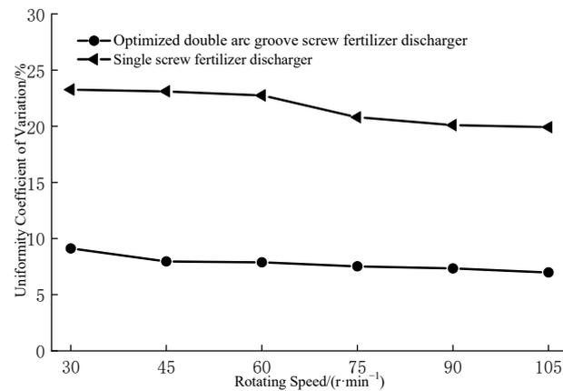
Figure 17. Uniformity coefficient of variation comparison test.
