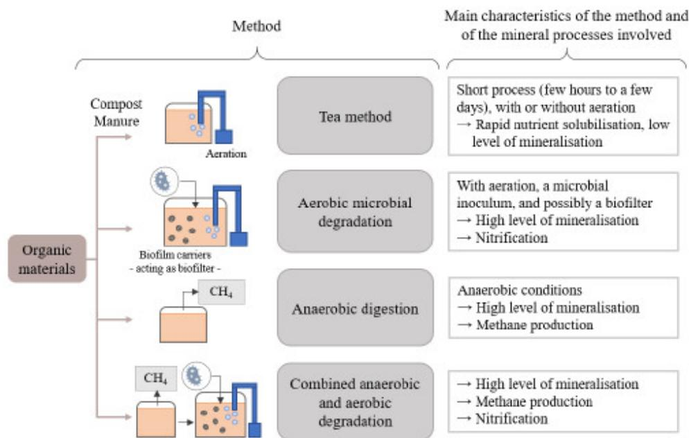
**Figure 1.** Overview of the most commonly used bioponic methods to produce nutrient solutions [8].
