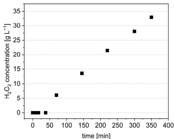
**Figure 5.** Electrochemical  $H_2O_2$  production in 0.5 M  $KHCO_3/K_2CO_3$  electrolyte at  $81 \text{ mA cm}^{-2}$ .
