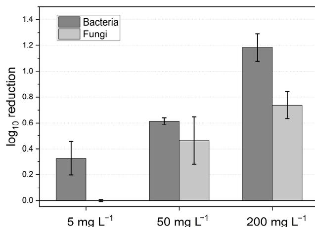
**Figure 7.** Log<sub>10</sub> reduction of bacteria and fungi for different concentrations of H<sub>2</sub>O<sub>2</sub> from ex situ electrochemical production compared to the control samples (no active H<sub>2</sub>O<sub>2</sub> ingredient) after an incubation time of 30 min under stirring conditions (Scenario C1–C3).
