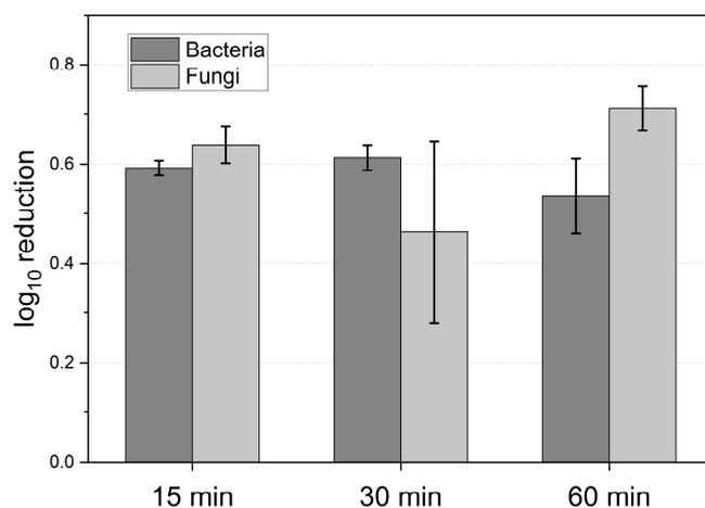
**Figure 8.** Log<sub>10</sub> reductions of bacteria and fungi for different reaction times of microorganisms with H<sub>2</sub>O<sub>2</sub> from ex situ electrochemical production compared to the control samples (no incubation time with H<sub>2</sub>O<sub>2</sub>), with an active ingredient concentration of 50 mg L<sup>-1</sup> under stirring conditions (Scenario R1–R3).
