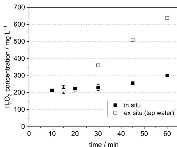
**Figure 6.** Ex situ H<sub>2</sub>O<sub>2</sub> production in tap water for subsequent dosing to the nutrient solution (open symbols) and in situ production directly in the nutrient solution (full symbols). The current density was approximately 6 mA cm<sup>-2</sup> for the ex situ and 16 mA cm<sup>-2</sup> for the in situ experiment.
