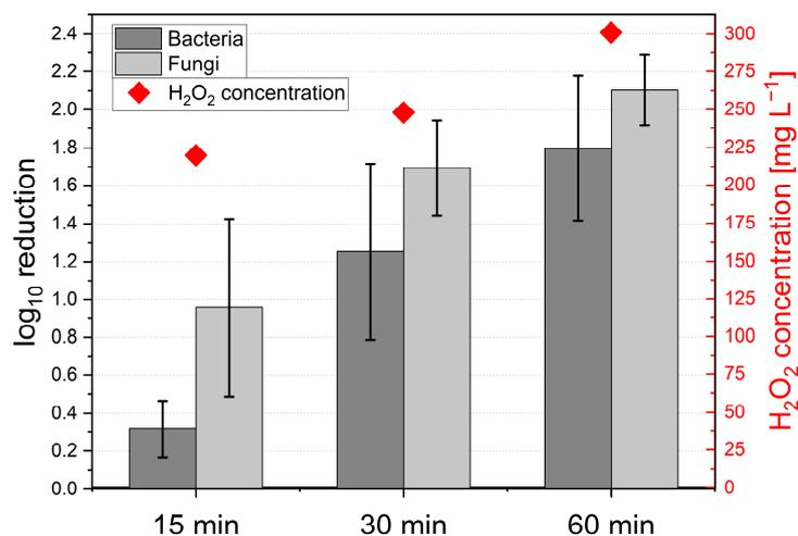
**Figure 9.** Log<sub>10</sub> reductions of bacteria and fungi for different in situ  $\text{H}_2\text{O}_2$  production times compared to the control samples (no in situ  $\text{H}_2\text{O}_2$  production) at a pump speed of  $25 \text{ L h}^{-1}$  and for a total nutrient solution of 500 mL. The red diamonds indicate the average final hydrogen peroxide concentrations after each production time interval (Scenario IS1–IS3).
