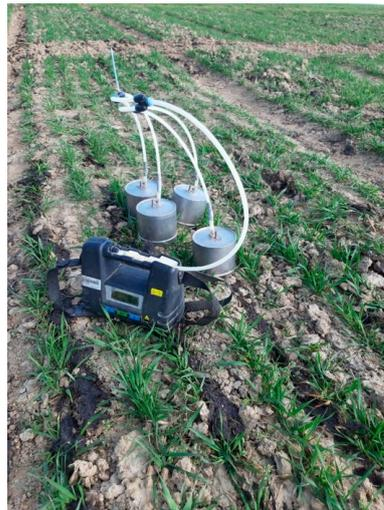
Figure A3. Ammonia measurement using the DTM method in a fertilised wheat plot.
