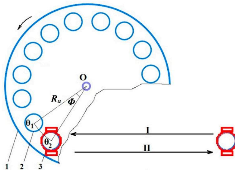
**Figure 3.** Aspects of distribution and planting movements: (1) distribution apparatus disc; (2) receiving tube; (3) planting device; I—return stroke; II—planting stroke;  $R_a$ —the radius of the distribution apparatus at the centers of the receiving tubes  $\Phi$ —the angle at the center corresponding to the arc  $\theta_1\theta_2$  described by the distribution apparatus disc for supplying a seedling to the planting device.
