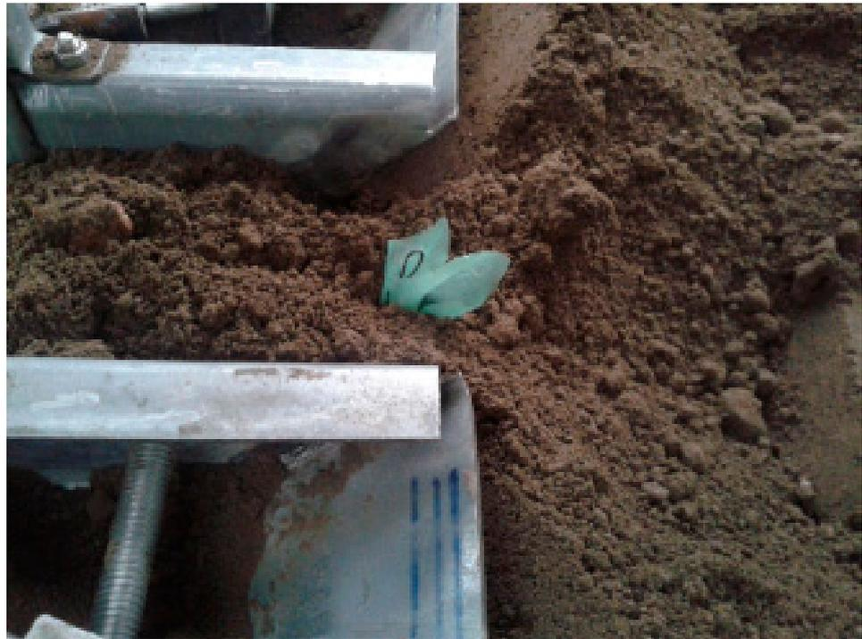
**Figure 23.** Tilted and partially buried seedlings in the winged skid-fixing process.
