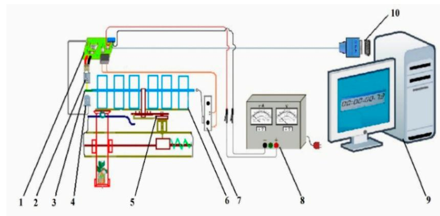
**Figure 6.** Installation diagram for measuring the distribution device permutation time: (1) data acquisition board; (2) infrared phototransistor; (3) shutter; (4) infrared LED; (5) ratchet system; (6) distribution apparatus; (7) micro-switch; (8) DC power supply; (9) computer; (10) serial port.
