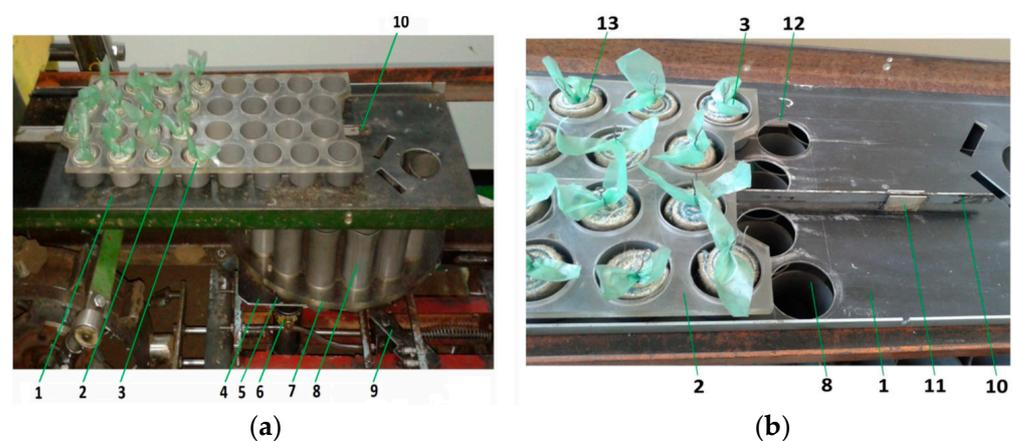
**Figure A2.** Seedling feeding system: (a) General view; (b) Alveolar seedling tray on feed table; (1) feed table; (2) alveolar tray; (3) current row of simulacra seedlings; (4) holding-release screen; (5) slot of the holding-release screen; (6) planting device; (7) distribution apparatus; (8) receiving tube of the distribution apparatus; (9) scotch-yoke mechanism; (10) push rod; (11) rod guide; (12) slots of the feed table; (13) simulacra seedling in growing cell.
