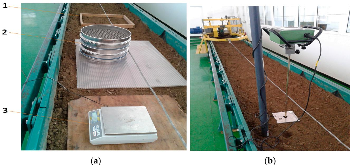
**Figure 13.** Aspects of the determinations of soil characteristics in the test bin: (a) soil particle size analysis: (1) metric scale; (2) soil sieves set; (3) precision balance; (b) penetration resistance and soil moisture determinations are cited.
