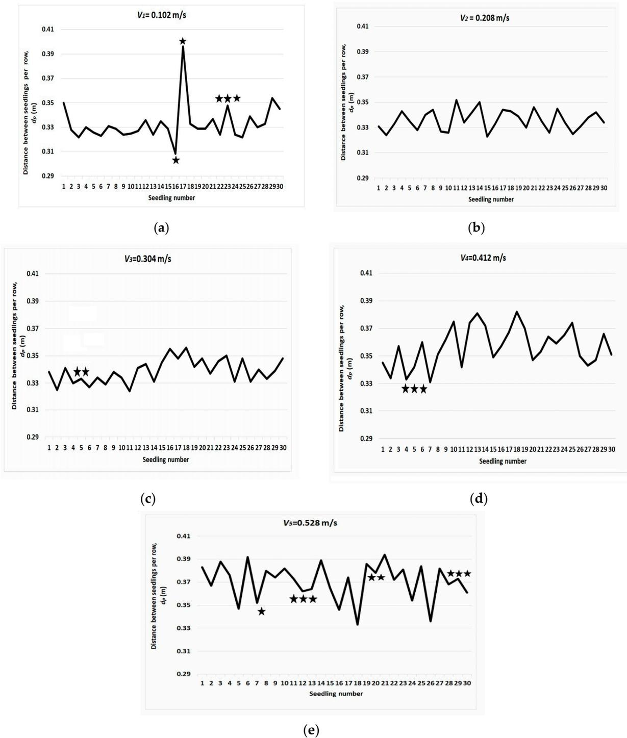
**Figure 16.** Distances measured between seedlings on the row. (a) Results for  $V_1$ ; (b) results for  $V_2$ ; (c) results for  $V_3$ ; (d) results for  $V_4$ ; (e) results for  $V_5$ . Errors due to: ★ distribution apparatus blockages, ★★ unfixed seedling, ★★★ wrongly planted seedling.
