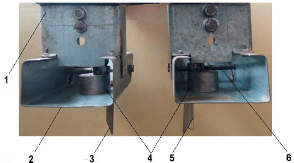
**Figure 22.** Winged fixing skids-rear view: (1) support; (2) active surface of the skid; (3) skid wing; (4) rotating hub for adjusting the distance between the skid wings; (5) the angle made by the wing with the forward direction; (6) device for adjusting the wing inclination angle with the direction of travel.
