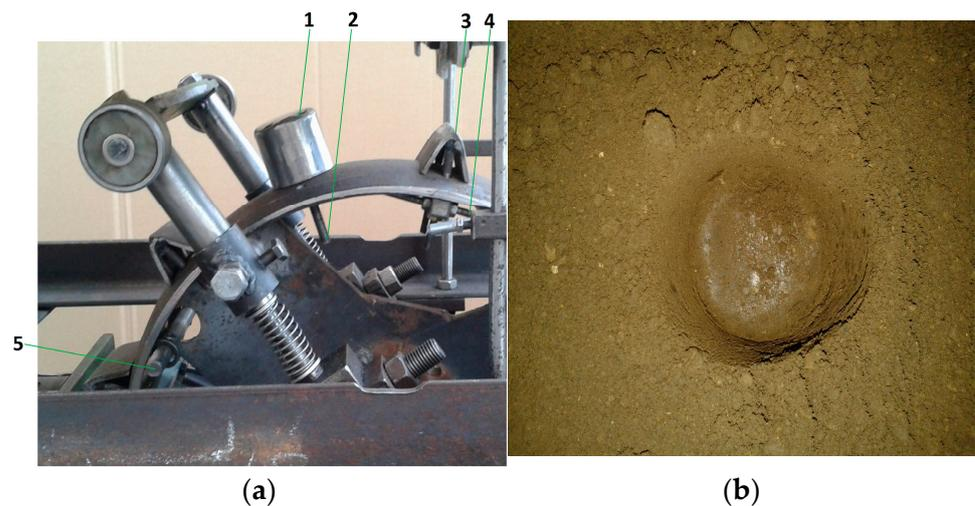
**Figure 21.** Influence of the spur's shape on the planting hole profile. (a) Detail of the planter wheel: (1) spur; (2) fixing and adjusting screw; (3) anti-slip profile; (4) threaded adjusting rod; (5) control rod. (b) Elongated planting hole.
