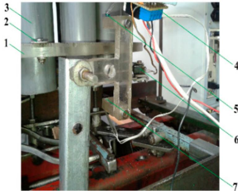
**Figure 10.** Installation configuration used to determine the distribution apparatus permutation time: (1) distribution apparatus disc; (2) receiving tube; (3) shutter; (4) acquisition data board; (5) Infrared LED; (6) micro-switch; (7) infrared phototransistor.
