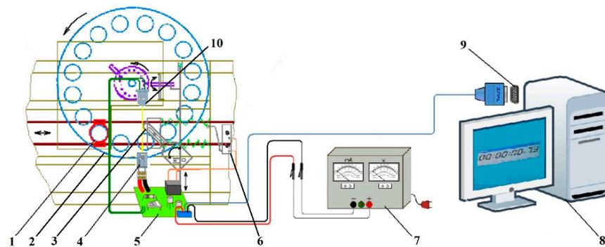
**Figure 5.** Installation diagram for measuring the return time of the planting device: (1) planting device; (2) distribution apparatus; (3) scotch-yoke device; (4) infrared phototransistor; (5) data acquisition board; (6) micro-switch; (7) DC power supply; (8) computer; (9) serial port; (10) infrared LED.
