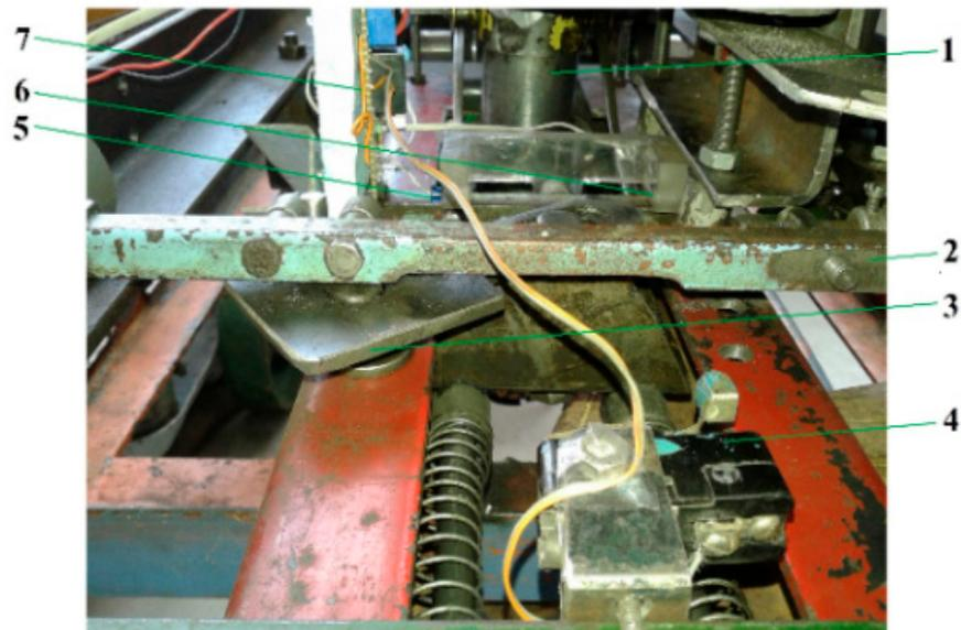
**Figure 9.** Installation configuration used to determine the return time of the planting device: (1) planting device; (2) oscillating sliding bar; (3) oscillating scotch-yoke lever; (4) micro-switch; (5) infrared LED; (6) infrared phototransistor; (7) data acquisition board.
