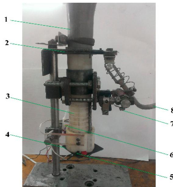
**Figure 12.** Auxiliary installation for seedling's fall time determination adjusted for the height of 228 mm: (1) receiving tube; (2) trapdoor; (3) planting device tube; (4) plate for stopping the seedling; (5) infrared phototransistor; (6) electronic device (with Infrared LED); (7) micro-switch; (8) lever.
