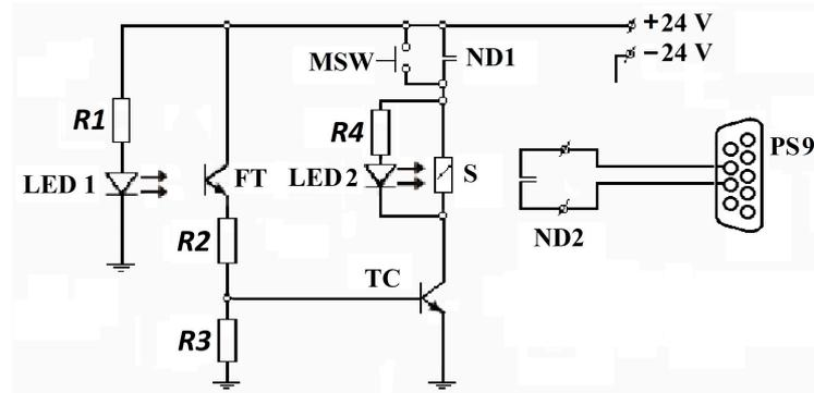
**Figure 4.** Electronic control block: R1—2 kΩ electrical resistance; R2—8 kΩ electrical resistance; R3—0.560 kΩ electrical resistance; R4—2 kΩ electrical resistance; LED 1—light in infrared emission; LED 2—light in infrared phototransistor; MSW—micro-contact; TC—control transistor; ND1—normally open contact; ND2—normally open contact; S—solenoid; PS9—PC nine-pin serial port.
