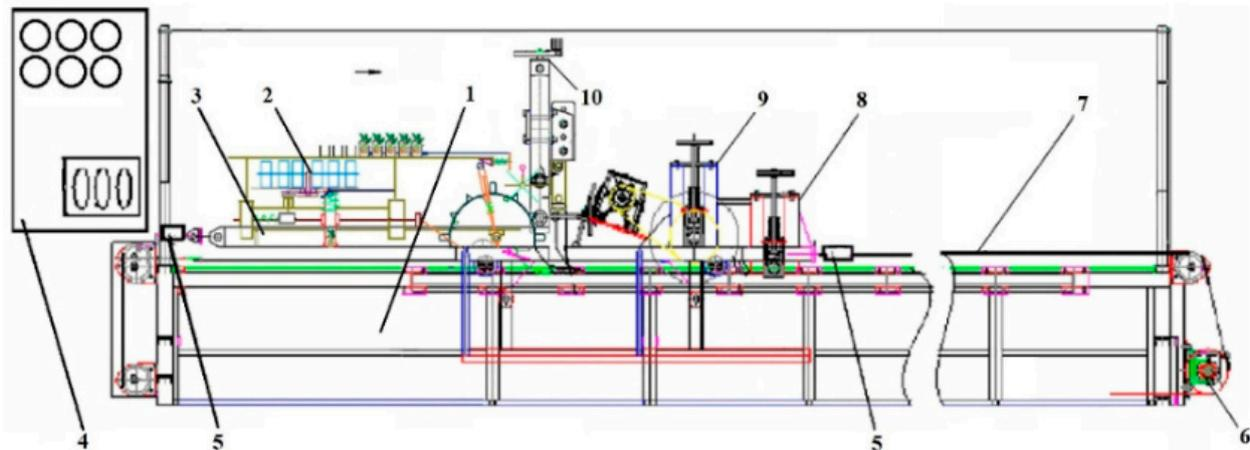
**Figure 8.** Soil bin test rig: (1) soil channel frame; (2) planting machine; (3) trolley; (4) control panel; (5) sensors for measuring the pulling force; (6) electric motor for driving the trolley; (7) pulling cable; (8) vertical loading mechanism on the roller; (9) vertical loading mechanism on the wheel; (10) mechanism for vertical adjustment of the machine's clamping support.
