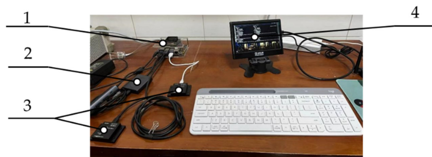
Figure 4. Test equipment. 1—NVIDIA Jetson Nano development board; 2—Green Union wireless projection device; 3—IMU attitude sensor; 4—MAKEBIT 4B display.
