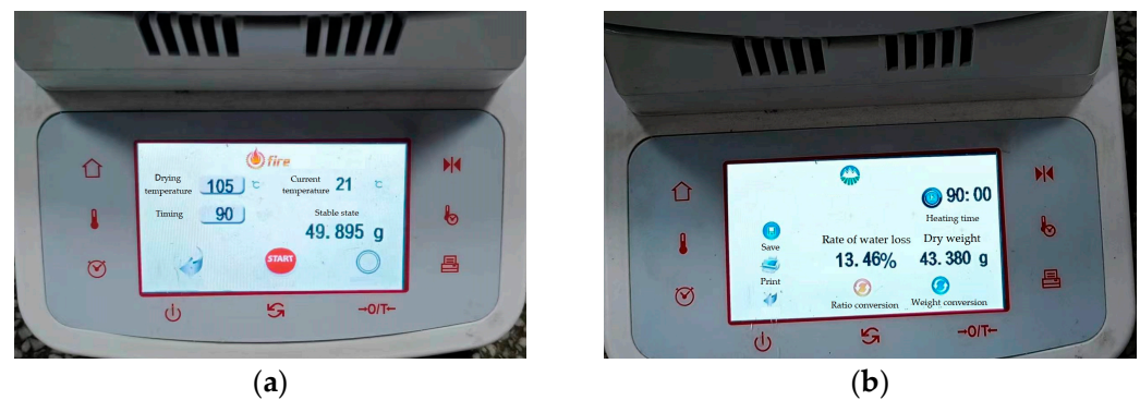
Figure 1. Determination of moisture content in maize kernels. The setting (a) and the result (b).
