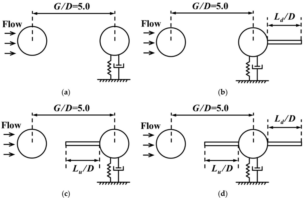
**Figure 1.** Diagram of the cylinder–plate body in different additional positions. (a) DC; (b) DCP; (c) DPC; (d) DPCP.
