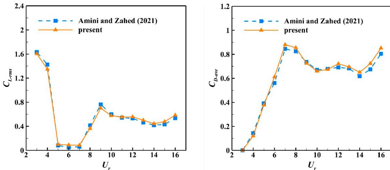
Figure 4. Verification results of the  $C_{L-rms}$  and  $C_{D-ave}$  of a cylinder–plate body against the reduced velocity  $U_r$  [26].
