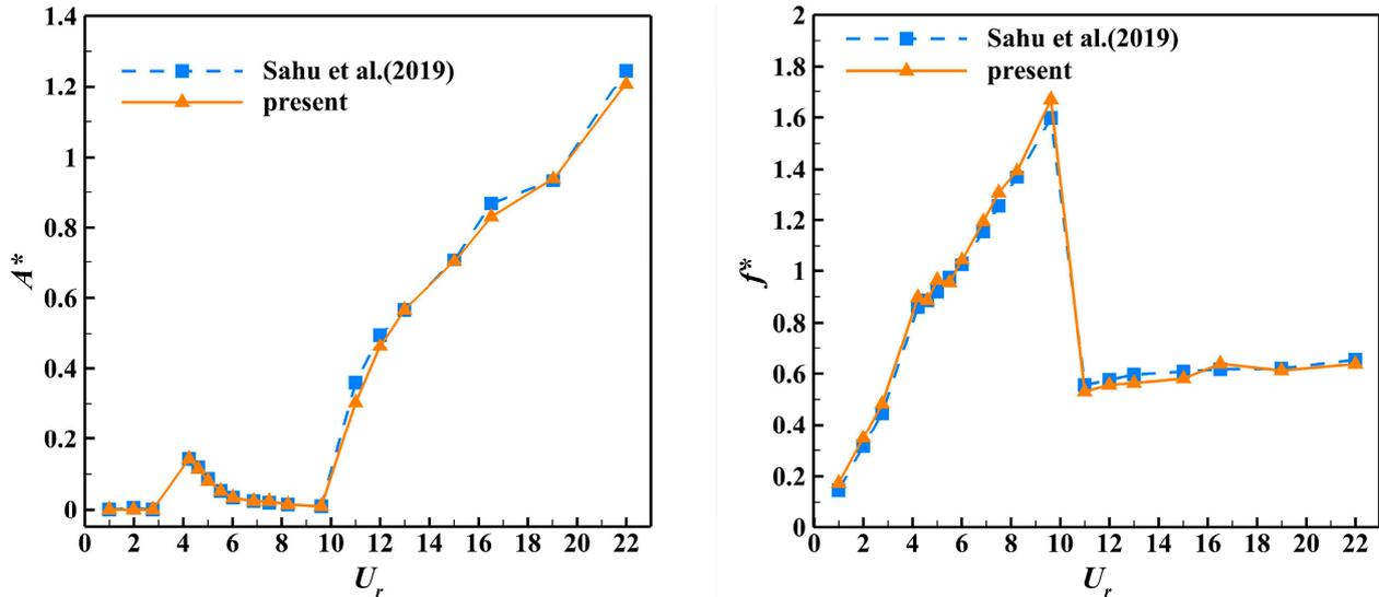
Figure 3. Verification results of  $A^*$  and  $f^*$  of a cylinder–plate body against the reduced velocity  $U_r$  [24].
