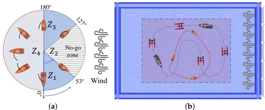
**Figure 7.** Points of sail and path examples. (a) Different sail modes have been adopted in different zones. The wind blows from the right-hand side. (b) There are two path examples. The darker rectangle represents the active sailing zone. The wind direction is from right side.
