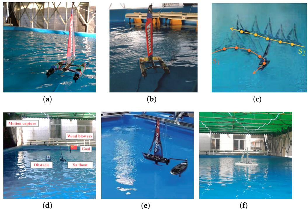
**Figure 15.** Previous works. (a) Automatic sailing with miniSailBot-B. (b) Automatic sailing with miniSailBot-C. (c) Collision avoidance by racing rule of sailing (RRS) with miniSailBot-D. (d) Collision avoidance by reinforcement learning (RL) with miniSailBot-D. (e) Enhanced autonomous sailboat with miniSailBot-D. (f) Station keeping with miniSailBot-E.
