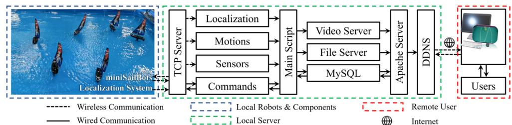
**Figure 4.** Internet server framework of STAR. The framework consists of local robots and devices, local server and remote users. The local server plays the part of connection between local robots and remote users.
