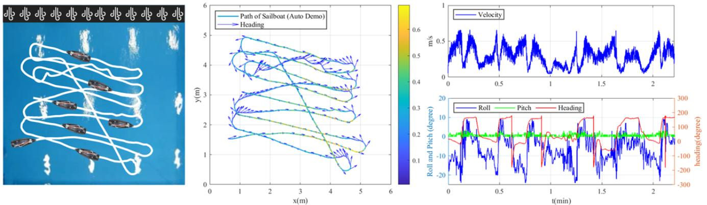
**Figure 12.** Automatic control in remote teaching mode. The left picture shows the path and wind direction in real test environment. The middle figure is the path of the sailboat with heading arrow and speed color-bar. The right figures are velocity and attitude versus time.
