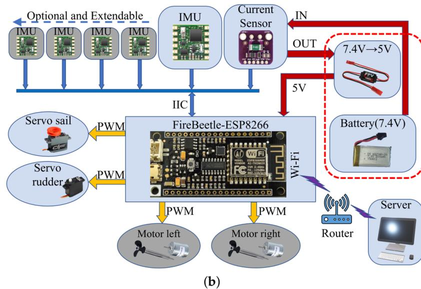
**Figure 2.** The miniSailBots and electronic hardware. (a) miniSailBots of different sizes. (b) Diagram of electronic hardware modification structure.
