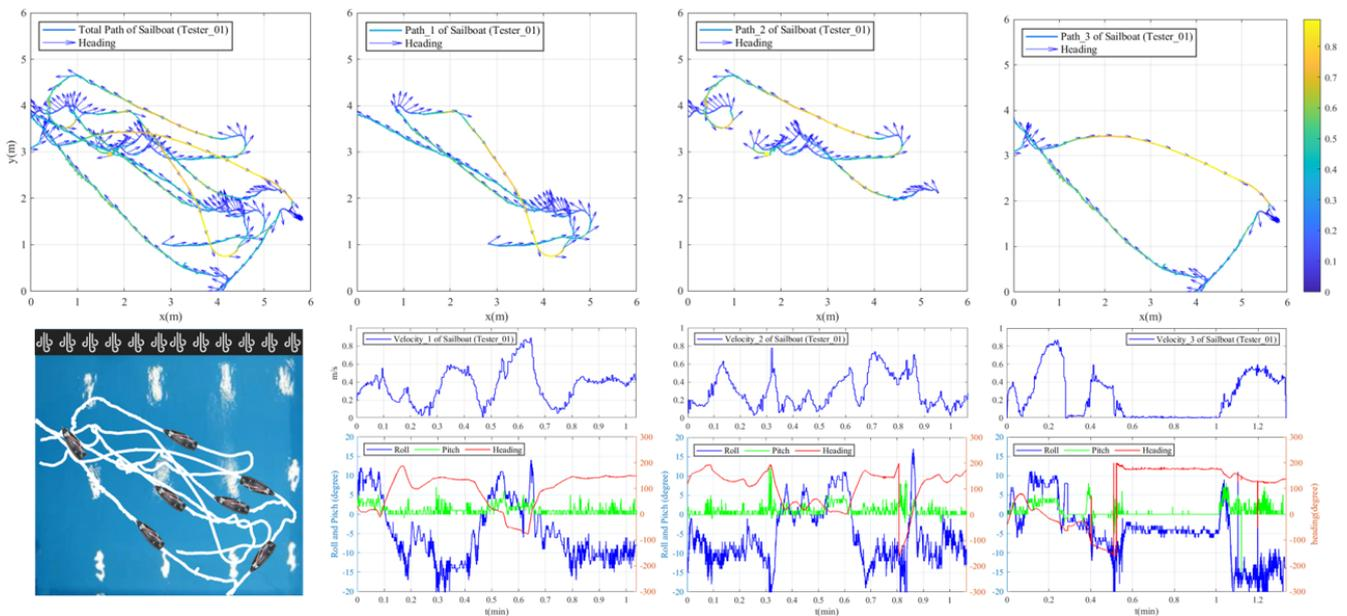
**Figure 9.** Remote sailing test (tester 01) in STAR. The leftmost figure of the first row and the remaining three figures are the total sailing path and the segmented paths, respectively. The arrow in the path indicates the heading. The graph in the second row is the path in the real test environment corresponding to the figure in the first row. The remaining three diagrams all contain the speed, roll, pitch and heading of the corresponding path.
