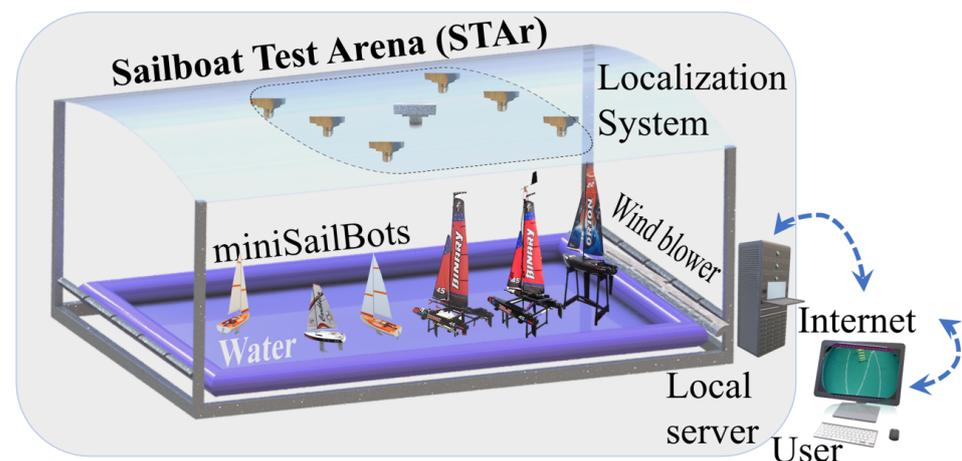
**Figure 1.** STAR architecture. The platform comprises of miniature sailing robots (miniSailBots), an arena including an 6 m (length)  $\times$  6 m (width) pool with 0.3 m depth water, a quasi controllable wind field, a localization system and a network server.
