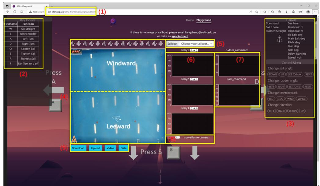
**Figure 5.** User interface of STAR. (1) The shared network address of STAR; (2) Key indices; (3) Information dashboard; (4) The pool region, wind direction, windward and leeward zones. (5) Selector for selecting a ready sailing robot. (6) Real-time display of delay. (7) Sail and rudder control commands. (8) Button for opening or closing the surveillance camera. (9) Buttons for remote algorithm deployment.
