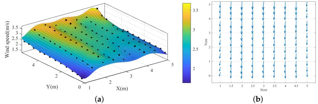
**Figure 3.** Wind field in STAR. (a) 3D wind field distribution. The black dots represent the monitoring sites. The color is used to show the magnitude of the wind speed. (b) display of wind direction and corresponding wind speed in the pool area.
