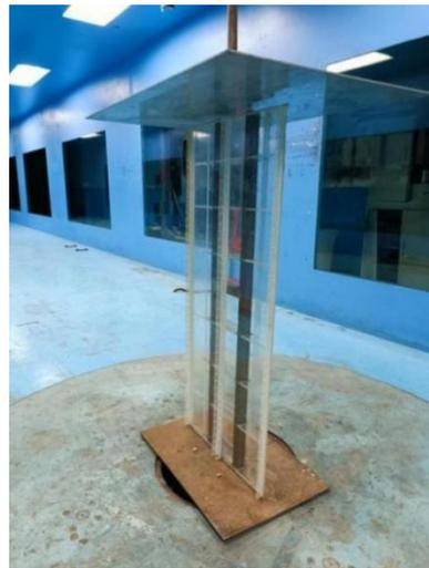
Figure 11. Segment model of the girder of the sea-crossing bridge in wind tunnel laboratory.
