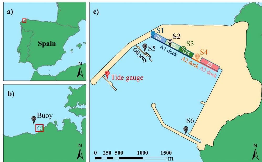
**Figure 1.** (a) Spain, showing the location of A Coruña, (b) situation of the port, buoy and zoom for section c, (c) plan view of the Outer Port of Punta Langosteira and position of pressure sensors (S1, S2, S3, S4, S5 and S6) and the tide gauge.
