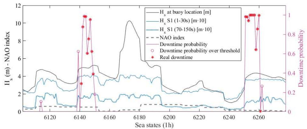
**Figure 10.** Time series of significant wave heights, NAO index, and downtime probability with real events.
