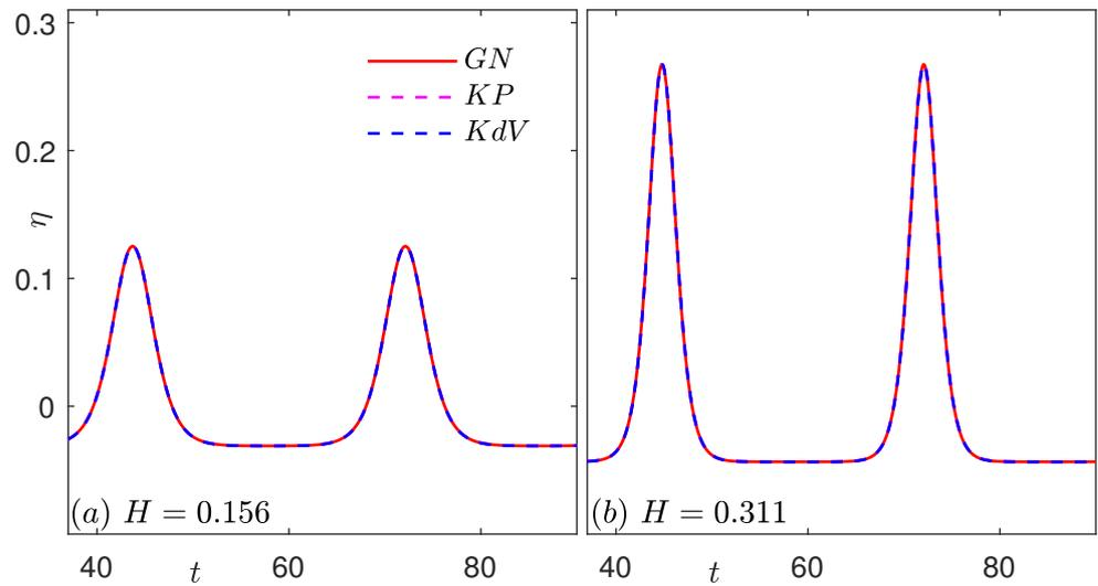
**Figure 3.** Comparisons of steady-state surface elevation of cnoidal waves generated by various theories.  $\lambda = 29.6$ .
