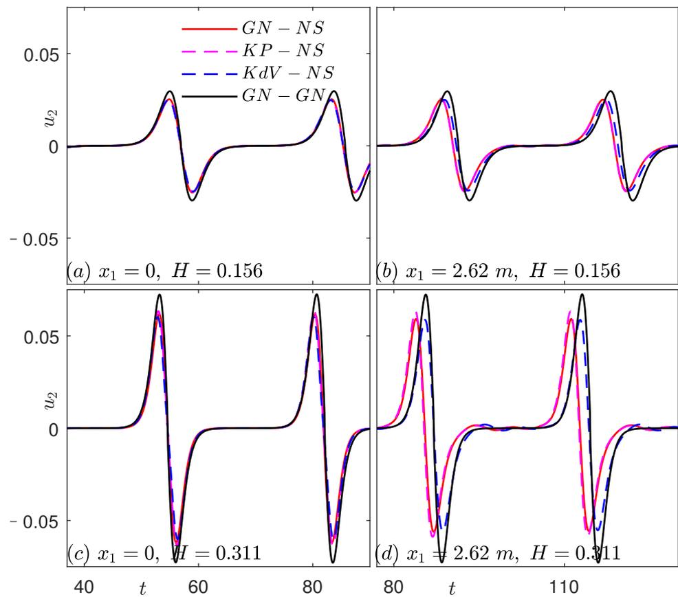
**Figure 13.** Comparisons of vertical particle velocity of cnoidal waves generated by various theories, propagating in domain of the NS equations.  $\lambda = 29.6$ .
