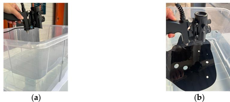
**Figure 3.** This figure shows the visual appearance of the different hydrocarbons used in this research. (a) Water hyperspectral signatures acquisition and (b) high-sulphur fuel oil hyperspectral signatures acquisition.
