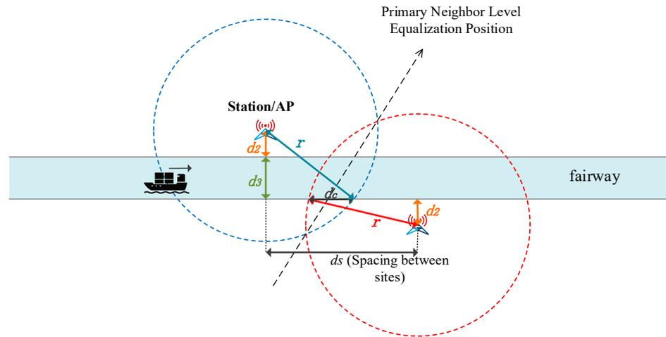
Figure 3. Overlapping coverage belt.
